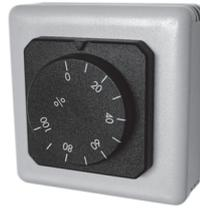
External Speed Control for the COOK EC Motor allows the fan speed to be adjusted remotely via an easy to read dial. The controller allows for adjustment from 20-100% of the fan speed. The controller works with the external signal version of the COOK EC Motor and requires 24 VAC power for operation. It is shipped loose for field installation.
