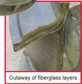
Cutaway of fiberglass layers
