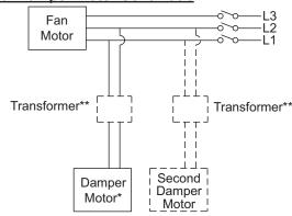
For 3 phase, damper motor voltage should be the same between  $L_1$  and  $L_2$ . For single phase application, disregard  $L_3$ . \*Damper motors may be available in 115, 230 and 460 volt models. The damper motor nameplate voltage should be verified prior to connection. \*\*A transformer may be provided in some installations to correct the damper motor voltage to the specified voltage.
